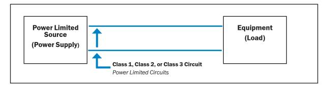
Most common is a Class 2 circuit, which offers protection for fire initiation and electric shock. For a 24VDC power supply (the most commonly used Class 2 voltage), the maximum power allowed is 100W. The power supply must be listed to applicable standards.
