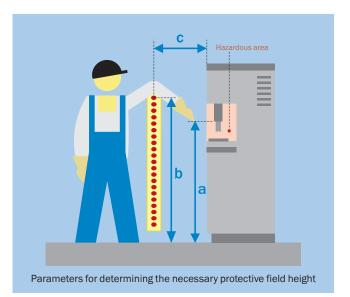
A special table for the necessary protective field height of ESPE was in preparation as in the new Draft of ISO 13855 at the time of going to press.
