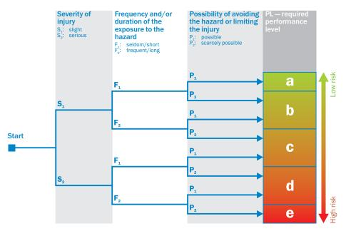
The performance level is defined in five discrete steps. It depends on the structure of the control system, the reliability of the components used, the ability to detect failures, as well as the
