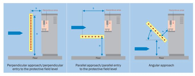
After the ESPE has been selected, the necessary safety distance between the ESPE's protective field and the nearest hazardous point is to be calculated.
