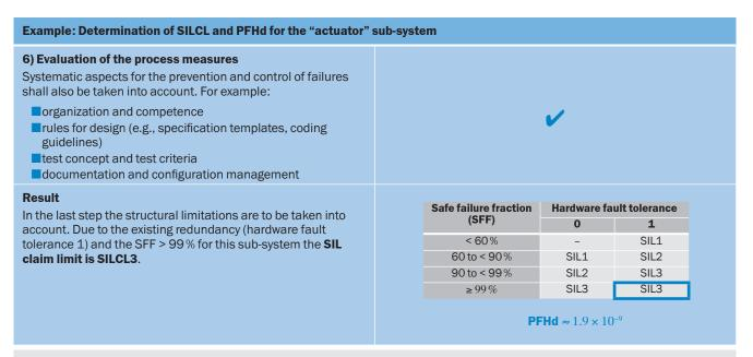
With the resulting SILCL data and the PFHd figure for the sub-system, the SIL achieved for the entire safety function can be determined as described above (see "Safety integrity of the hardware" on page 3-59).
