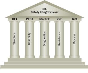
The safety integrity level (SIL) achieved for a sub-system comprises the following parameters:
