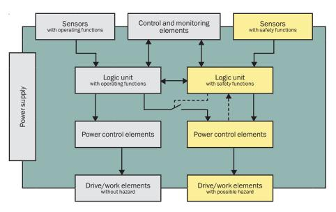
The safety-related parts of control systems are to be selected to suit the safety functions and the necessary safety performance e.g. sensors, logic units, power control elements as well as drive and work elements. This selection is generally made in the form of a safety concept.
