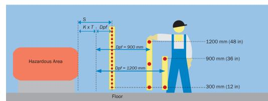
Example of guarding with various detection capabilities for the perpendicular approach
