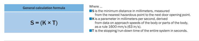
Calculation of the safety distance for interlocked physical guards: ANSI B11.19, ISO 13855
