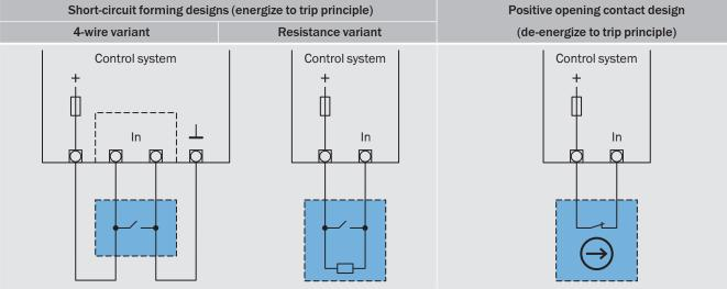
Here a short-circuit is formed on the activation of the protective device. In the case of the 4-wire version, a circuit is short-circuited (a few Ohm). In the case of the resistance variant, a change from a set resistance (in the kOhm range) is detected. These designs require more complex evaluation.
