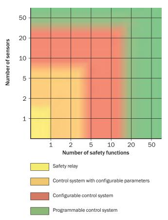
The functionality of the logical operators — e.g., simple AND, flipflop or special functions such as muting — also affects the selection.
