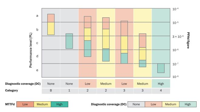
A performance level "d" can, e.g., be realized using a dual-channel control system (category 3). This can be achieved using good quality components (MTTFd = medium) if almost all failures are detected (DC = medium) or it is achieved with very good quality components (MTTFd = high) if a large number of failures are detected (DC = low). Behind this procedure there is a complex mathematical model of which the user is unaware.
