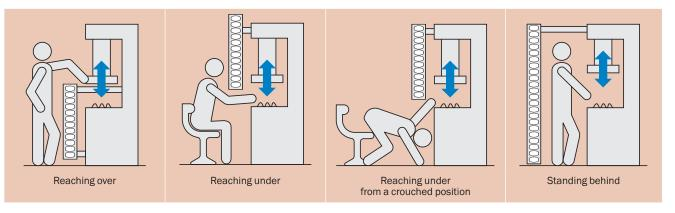
Once the minimum safety distance between protective field and the nearest hazardous point has been calculated, the protective field height required is to be determined in a further step. In this way it is to be ensured the hazardous point cannot be reached by reaching over.
